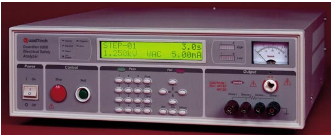
Figure 1: Guardian 6000 Series Electrical Safety Analyzer
